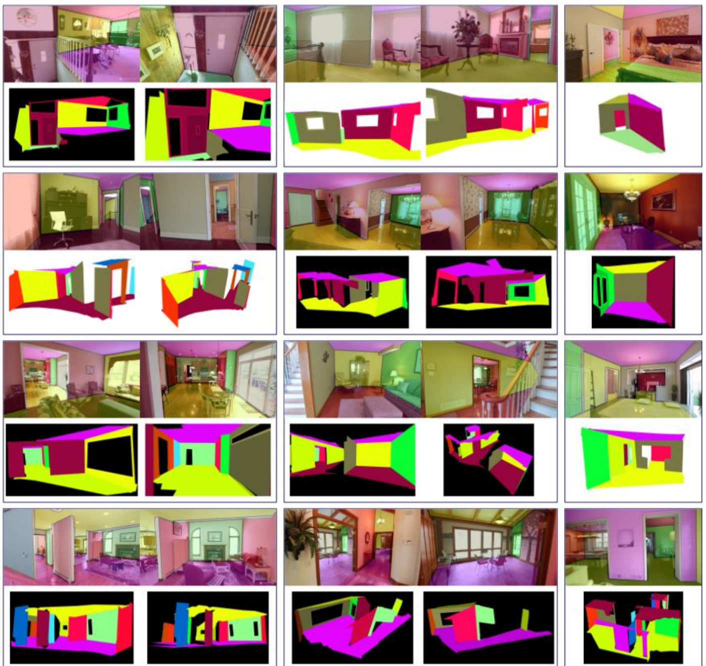
Figure 6: 3D Room layout reconstruction examples. For each example scene, we show one or two of the input annotations overlaid on the video frame (top), and the final reconstructed layout (bottom).
