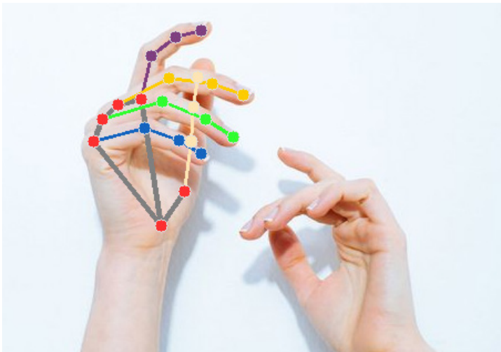
Figure 1: Result of Hand Tracking pipeline when using parameter min_detection_confidence set to 0.7
