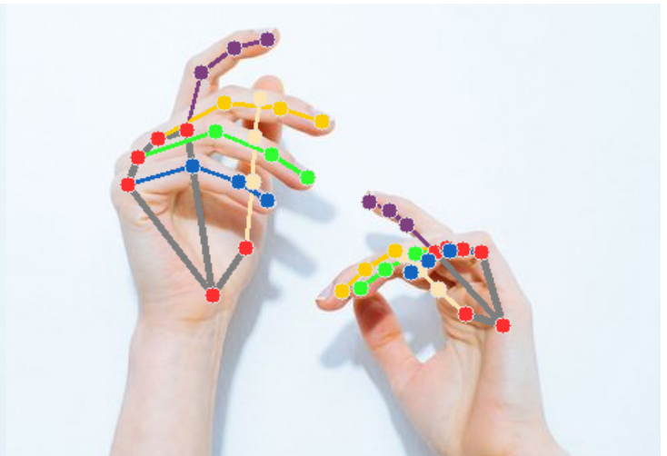
Figure 2: Result of Hand Tracking pipeline when using parameter min_detection_confidence set to 0.5
